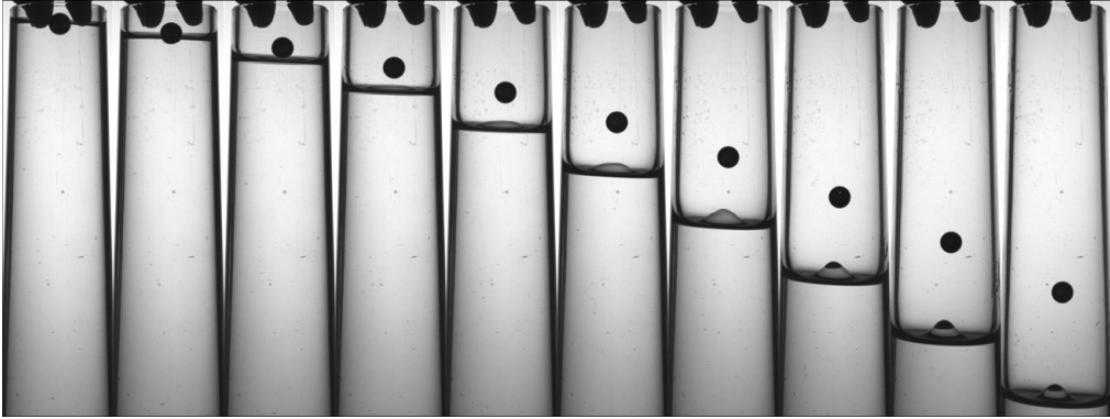
FIGURE 1. Free fall of a steel ball, and comparison with the position of the liquid interface in Tube 1, with ethanol. The pictures are equally spaced in time.
